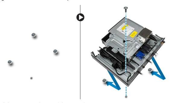
7. Install the antenna to the optical drive console.
